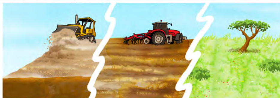
Replacing the overburden and topsoil
